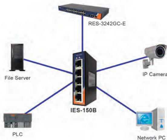
Connections of Ethernet devices
