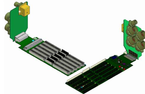
The customized backplane and the I/O transition board are designed using the same I/O signal characteristics, ensuring full matching of controlled impedances and signal integrity.
